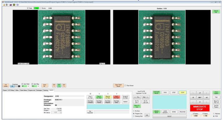
**Ideal for Inspecting:** Part Presence, Rotation, Polarity, Registration, Text, Solder, Solder Paste, Bent Leads, Bent Pins, Jumpers, Cut Traces, or any other top-down visual feature on the PCBA.
