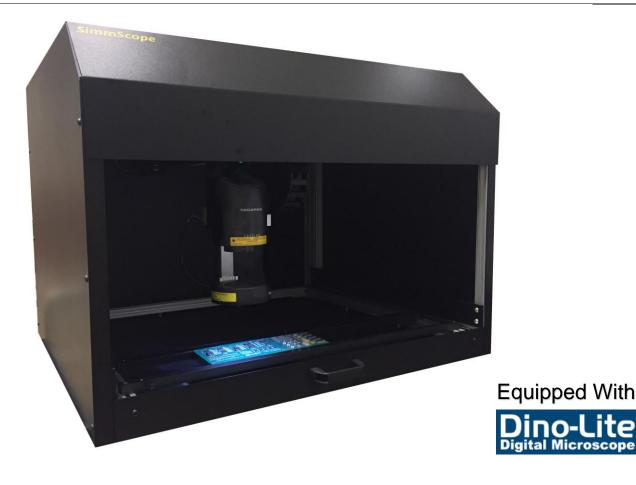
**The SimmScope SS-D** is an optical inspection and photo-documentation system for printed circuit board assemblies. It combines a **Dino-Lite** digital microscope with a computer controlled overhead XY positioner to automatically move the Microscope to visual inspection locations or image capture locations of the circuit board. The circuit board is placed into a board holder that is mounted inside a pullout drawer.
