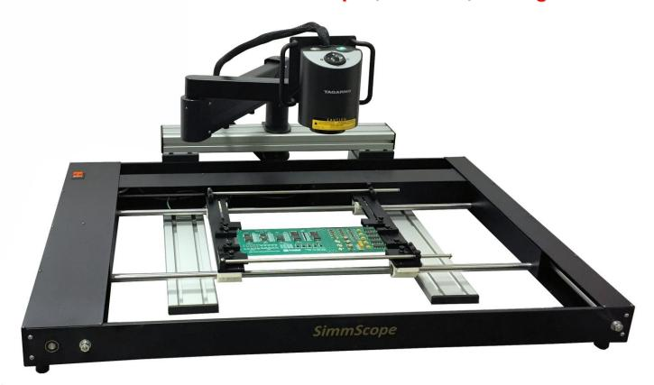
**The SimmScope SSXY** is an optical inspection and photo-documentation system for printed circuit board assemblies. It combines almost **any USB digital microscope or camera** with a computer controlled XY table to automatically move a circuit board to visual inspection locations or image capture locations to be viewed under the microscope. The circuit board can also be left in place while performing certain rework operations.
