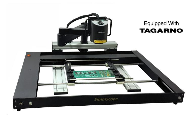
**The SimmScope SSXY-T** is an optical inspection and photo-documentation system for printed circuit board assemblies. It combines a **TAGARNO ZAP** digital microscope with a computer controlled XY table to automatically move a circuit board to visual inspection locations or image capture locations to be viewed under the microscope. The circuit board can also be left in place while performing certain rework operations.
